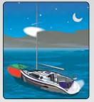
The masthead light and sternlight may be combined as an all-round white light on vessels less than 39.4 feet long.
